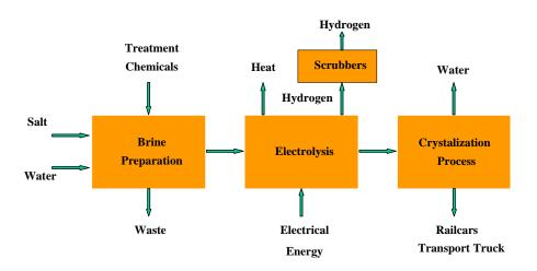
The sodium chlorate solution produced is treated and filtered to remove impurities and crystallized by removing excess water. Once cooled, the final product resembles a white crystal that is transported to customers by rail car, truck, pipeline or is bagged and shipped to international customers. ERCO Worldwide exports sodium chlorate from its Vancouver, British Columbia and Buckingham, Quebec production facilities.
