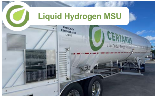
Certarus' first liquid hydrogen MSU
