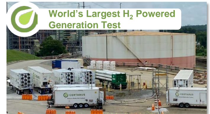
Provided on-site H 2 delivery to support the gas turbine fuel blending test with Mitsubishi at Georgia Power's Plant
