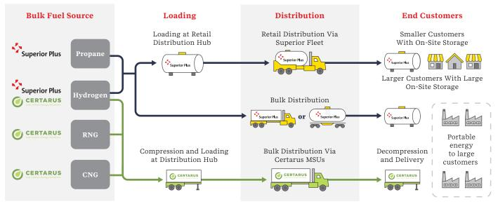
MSUs are interchangeable between CNG, RNG and hydrogen
