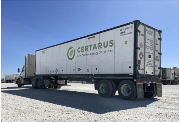
Large Volume CNG/RNG/Hydrogen MSUs – Trailered mobile storage units capable of delivering high volumes of gas payload
